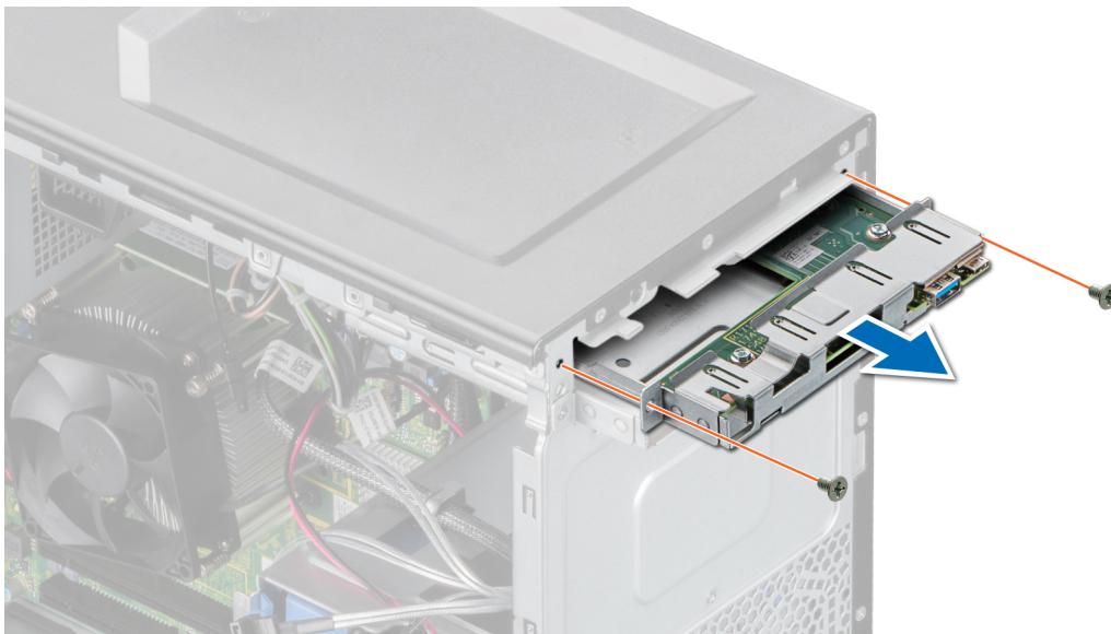
Figure 54. Removing the control panel cage
