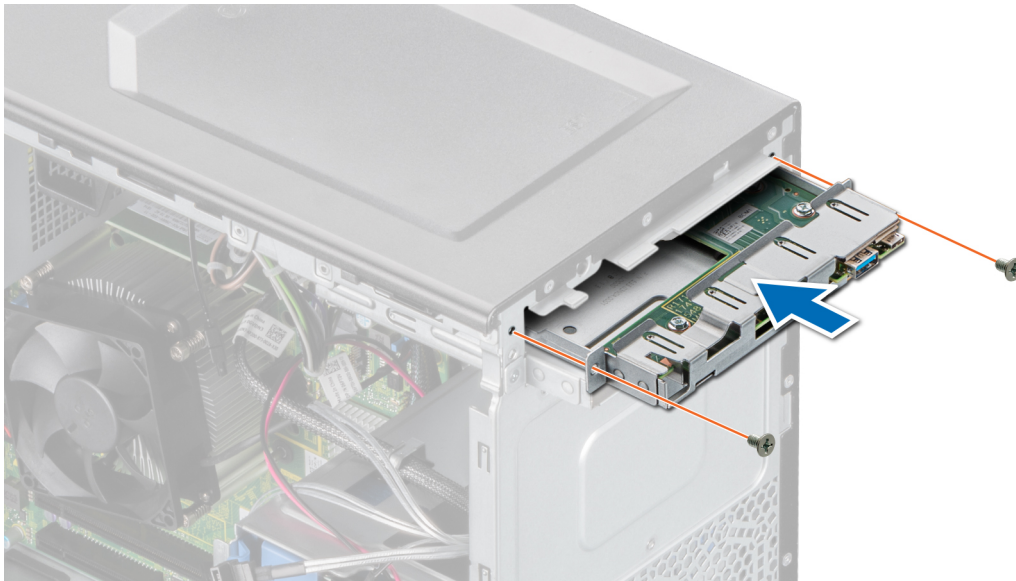
Figure 57. Installing the control panel cage
