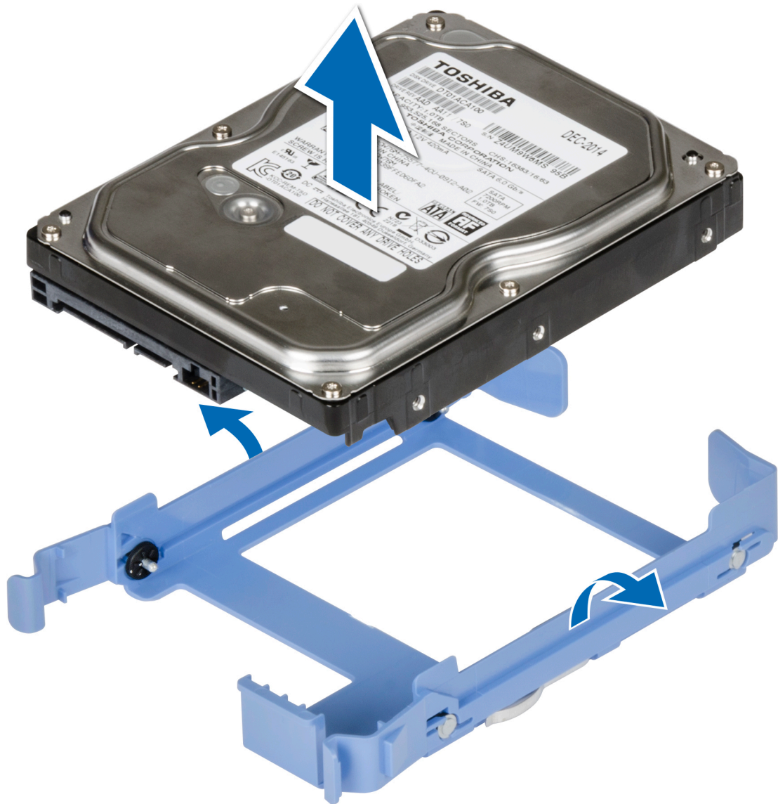
Figure 15. Removing the drive from the drive carrier
