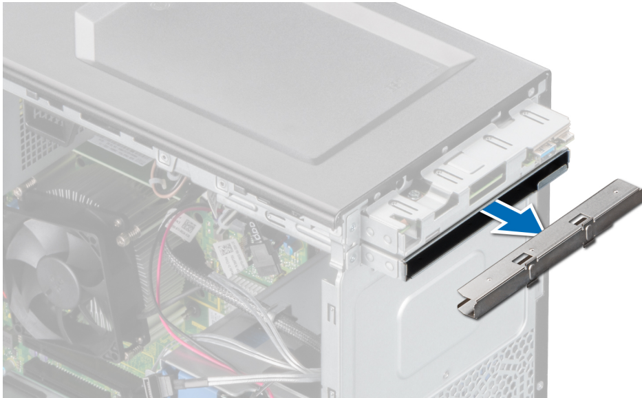
Figure 18. Removing the optical drive filler from the optical drive cage
